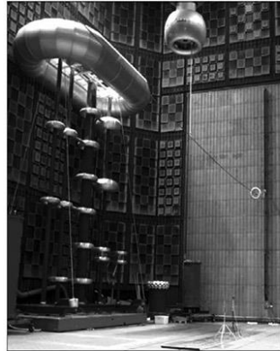
Figure 4) laboratory set-up of the single conductor measurement
